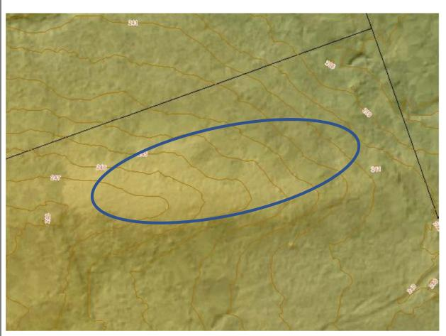
Infiltration gallery within the pond was removed and an alternate location is proposed on the east limits (east of ST-3) in order to ensure the gallery is not influenced by the water table, refer to the General Servicing Plan, CSP-1. This area does not cu-in as deep into the original ground significantly. Efforts can be made to further raise the gallery at detailed design to further reduce the risk of impact from the groundwater table.
