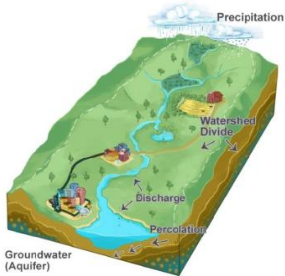
Figure 1 - A simple watershed with the boundary determined at the watershed divide
