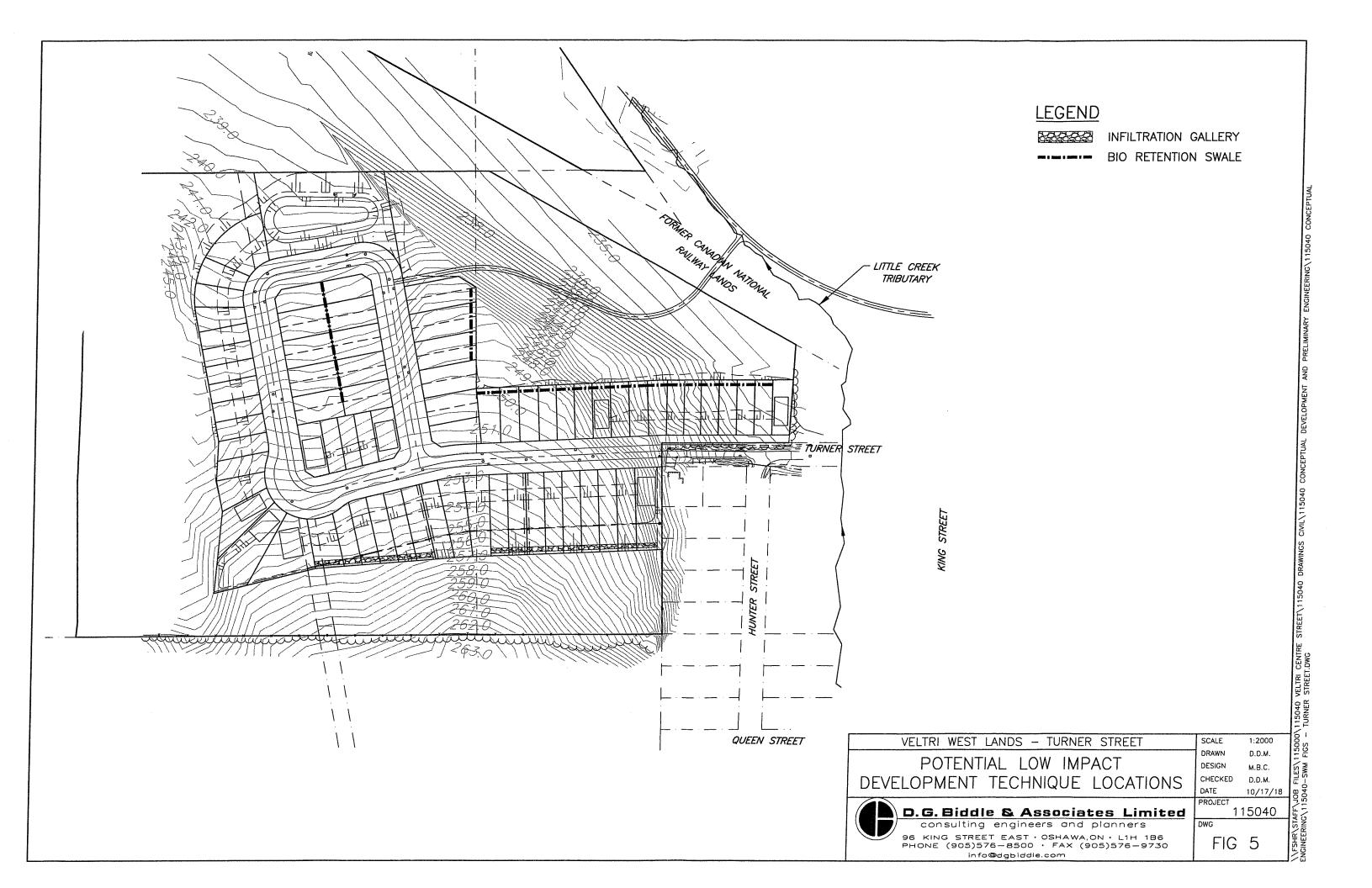
contributing area. Conceptual locations for the bio-retention swales are illustrated in Figure 5, with a detail provided on Figure 6. The suitability of these locations will need to be verified at the detail design stage.
