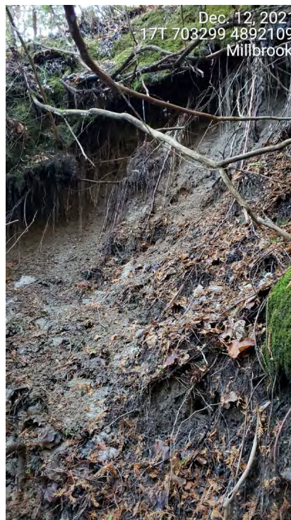
Photo 4 - Area of erosion of former rail line (south of residential area). Light brown silty sand observed. No rail ballast or discoloured soils noted.
