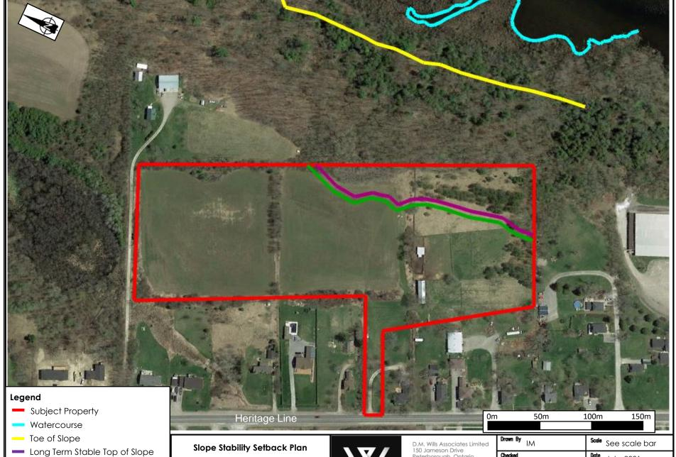
LTSTOS with 6m Erosion Access Allowance
